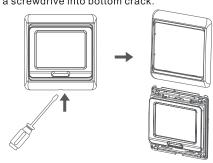
Take the backing plate apart according to the following diagram.
