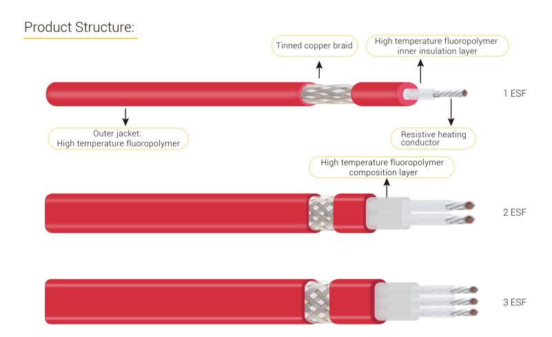
The core is resistive heating conductor, and high temperature fluoropolymer inner insulation layer, tinned copper braid, high temperature fluoropolymer are to be added to form a complete structure of ESF heating cable, in addition there is high temperature fluoropolymer composition layer between braid and conductor in twin-core (2ESF) and triple-core (3ESF) structure.
