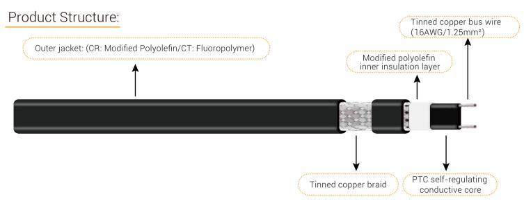
The extruded core tape, which made by parallel tinner copper bus wire and PTC semiconductor polymer heating material, and inner insulation layer of modified polyolefin are added to tinned copper braid and the outer jacket form a complete structure of HTLe heating cable, in which the outer jacket can be made of modified polyolefin material (CR) or fluoropolymer material (CT) according to different application or area.
