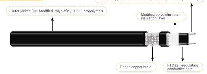
The extruded core tape, which made by parallel tinner copper bus wire and PTC semiconductor polymer heating material, and inner insulation layer of modified polyolefin are added to tinned copper braid and the outer jacket form a complete structure of HTR heating cable, in which the outer jacket can be made of modified polyolefin material (CR) or fluoropolymer material (CT) according to different application or area.
