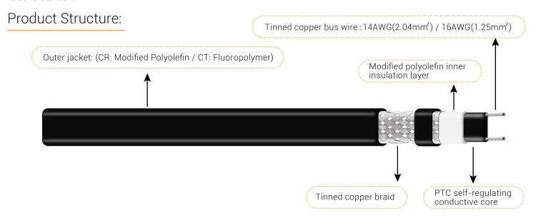
The extruded core tape, which made by parallel tinner copper bus wire and PTC semiconductor polymer heating material, and inner insulation layer of modified polyolefin are added to tinned copper braid and the outer jacket form a complete structure of HTR heating cable, in which the outer jacket can be made of modified polyolefin material (CR) or fluoropolymer material (CT) according to different application or area.
