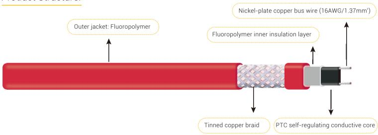
The extruded core tape, which made by parallel nickel-plate copper bus wire and PTC semiconductor polymer heating material, and inner insulation layer of fluoropolymer are added to tinned copper braid and the outer jacket form a complete structure of HTS heating cable, in which the outer jacket can be made of fluoropolymer material (CT).
